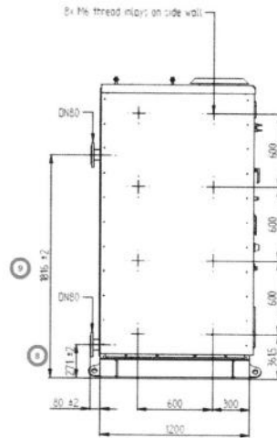
Figure 1-4: Converter Cabinet Side View
