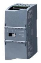
SIPLUS S7-1200 SM 1231 8AI based on 6ES7231-4HF32-0XB0 with conformal coating, -20...+60  $^{\circ}$ C, analog input SM 1231, 8 AI, +/-10 V, +/-5 V, +/-2.5 V, or 0-20 mA/4-20 mA, 12 bit+sign or (13 bit ADC)
