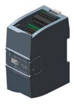
SIPLUS S7-1200 SM 1231 4AI 13 bit based on 6ES7231-4HD32-0XB0 with conformal coating, -20...+60  $^\circ C$ , analog input, 4 AI, +/-10 V, +/-5 V, +/-2.5 V, or 0-20 mA 12-bit+ sign bit (13 bit ADC)
