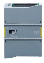
SIPLUS S7-1200 SM 1226 F-DQ 2x relay based on 6ES7226-6RA32-0XB0 with conformal coating, -25...+55  $^\circ$ C, F-DQ 2x RLY 5A, PROFIsafe, 70 mm width, up to PL e (ISO 13849-1)/ SIL3 (IEC 61508)
