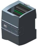
SIPLUS S7-1200 SM 1223 16DI/16DQ based on 6ES7223-1BL32-0XB0 with conformal coating, -40...+70  $^{\circ}$ C, start up -25  $^{\circ}$ C, digital input/output 16 DI/16 DQ, 16 DI 24 V DC, sink/source, 16 DQ, transistor 0.5 A
