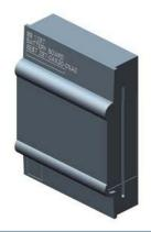
SIMATIC S7-1200, Battery Board BB 1297 for long-term buffering of the real time clock, plug-in in the signal board receptacle of the S7-12XX (FW3.0 or higher); Battery (CR1025) not included in scope of delivery
