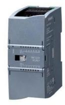
SIPLUS S7-1200 SM 1223 8DI/8DQ T1 rail based on 6ES7223-1BH32-0XB0 with conformal coating, -25...+55 °C, OT1 with ST1/2 (+70 °C für 10 minutes), digital input/output SM 1223, 8 DI/8 DQ, 8 DI 24 V DC, sink/source, 8 DQ, transistor 0.5 A
