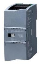
SIPLUS S7-1200 SB 1223 2DI/2DQ T1 rail based on 6ES7223-0BD30-0XB0 with conformal coating, -25...+55 °C, OT1 with ST1/2 (+70 °C für 10 minutes), digital input/output 2 DI 24 V DC/2 DQ 24 V DC
