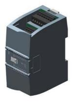
SIPLUS S7-1200 SM 1221 16DI based on 6ES7221-1BH32-0XB0 with conformal coating, -40...+70 °C, start up -25 °C, digital input 16 DI, 24 V DC, sink/source
