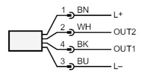
OUT1: switching output or IO-Link
