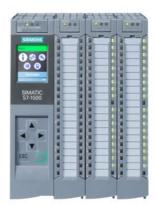
SIMATIC S7-1500 Compact CPU CPU 1512C-1 PN, central processing unit with working memory 250 KB for program and 1 MB for data, 32 digital inputs, 32 digital outputs, 5 analog inputs, 2 analog outputs, 6 high speed counters, 4 high speed outputs for PTO/PWM/frequency output 1. interface: PROFINET IRT with 2 port switch, 48 NS bit-performance, incl. front connector push-in, SIMATIC memory card necessary
