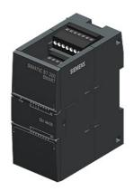
SIMATIC S7-200 SMART, analog I/O SM AM06, 4 AI/2 AO, 0..10 V, 0..5 V, 0/4..20mA, +/-5 V, +/-2.5 V, 12 bit resolution or 4...20 mA, +/-10 V 11 bit resolution
