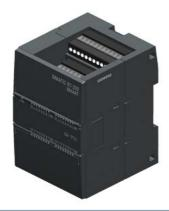
SIMATIC S7-200 SMART, Digital I/O SM DT32, 16DI/16DO, 16 DI 24 V DC, Sink/Source, 16 DO, Transistor 0.75A
