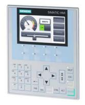
SIMATIC HMI KP400 Comfort, Comfort Panel, key operation, 4" widescreen TFT display, 16 million colors, PROFINET interface, MPI/PROFIBUS DP interface, 4 MB configuration memory, Windows CE 6.0, configurable from WinCC Comfort V11
