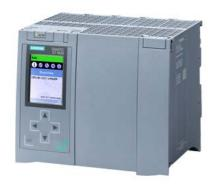
SIMATIC S7-1500, CPU 1517-3 PN/DP, Central processing unit with work memory 2 MB for Program and 8 MB for data, 1st interface: PROFINET IRT with 2-port switch, 2nd interface: PROFINET RT, 3rd interface: PROFIBUS, 2 ns bit performance, SIMATIC Memory Card required
